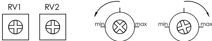
Warning: To use anti-crush function (recommended for small gates), it is necessary to regulate first the engine's power with the trimmer RV2 and right after the sensitivity with trimmer RV1. If you change the engine's power after performing a Working Time and Engine Pause programming , a new one is going to be needed.
