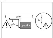
01. Position the operator 50 mm from the edge of the gate and perfectly square at an angle of 90° and mark the place to make the holes for the bushings. Must make the mark at the center of the oval holes
