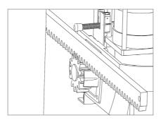
03. Mesh the rack with the pinion, leaving 1 to 2 mm backlash between the teeth. This backlash must remain constant over the entire length of the rack. Fix / weld the rack to the gate.
