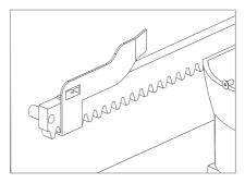
03. Bring the gate to its open position manually, stopping at a distance of 3cm from the mechanical limit stop. Slide the limit stop bracket along the rack until causing the limit stop to trip. Fix the bracket to the rack with the dedicated screws.Perform the same operation for the closing limit stop.
