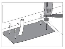
02. Drill four holes with Ø18mm on foundation. Place M10 steel anchors on the holes. Align it parallel to the gate leaving a distance of 50 mm and anchor the operator.
